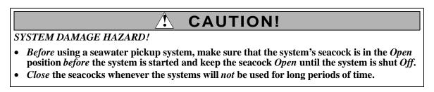
A seacock is a valve, controlled by a 90° lever, used to manage the pickup of seawater through the hull and below the water line. Seacocks are typically used on your boat in the following seawater pickup systems:
