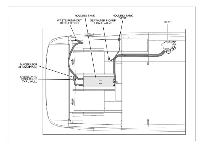
To use the macerator to pump waste directly into the water (where regulations permit):
