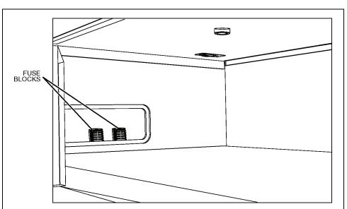
**12-Volt DC Fuse Blocks:** Located in the starboard wall hatch in the aft berth.
