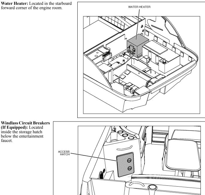
Windlass Circuit Breakers (If Equipped): Located inside the storage hatch below the entertainment faucet.
