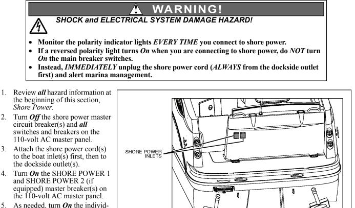
5. As needed, turn **On** the individual component breakers on the 110-volt AC master panel.
