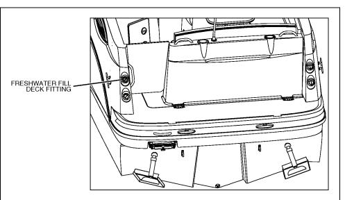
Freshwater Fill Deck Fitting (marked WATER): Located on the port aft corner of the deck.
