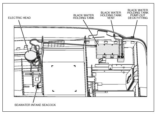
• Keep the intake seacock *Closed* while your boat is underway or when the system will not be used for long periods of time.
