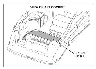
The bilge blowers remove fumes from the engine compartment and draws fresh air into the compartment through the deck vents. To ensure fresh air circulation, operate the bilge blowers for at least four minutes prior to starting the engines (or optional generator), during starting, and while operating your boat below cruising speed.
