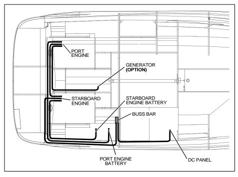
Negative Battery Cable Harness (Diesel Option)
