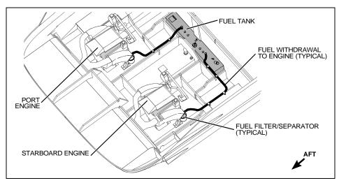
Diesel Fuel System Routing (Option)
